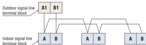
o Indoor and outdoor signal lines do not have a polarity. Any of the connections in the following illustration can be made.
