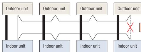
The signal lines cannot form a loop, so the wirings shown as ..... in the diagram are prohibited.
