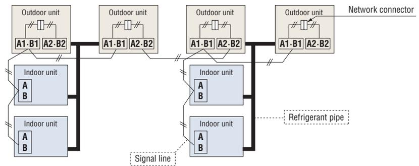
The maximum number of indoor units that can be connected in a system is 128 and it is possible to configure outdoor units and/or indoor units as an outdoor or indoor unit group connected with each other with two wires.
