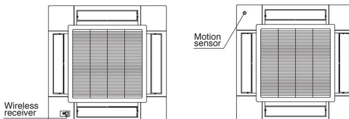
\*Wireless receiver and Motion sensor can be installed to the position as shown
