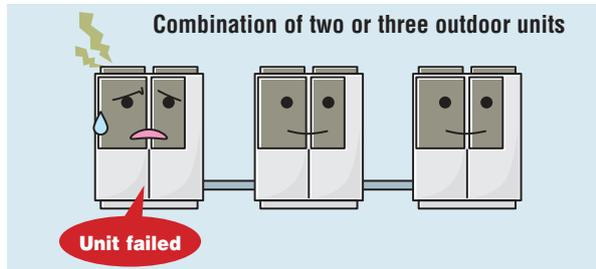
In the event that one compressor has a failure, the unit will keep operating with the another good compressor.
