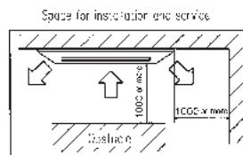
Make a space of 400mm or more between the units when installing more than one.
