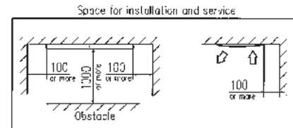
Make a space of 400 or more between the units when installing more than one.
