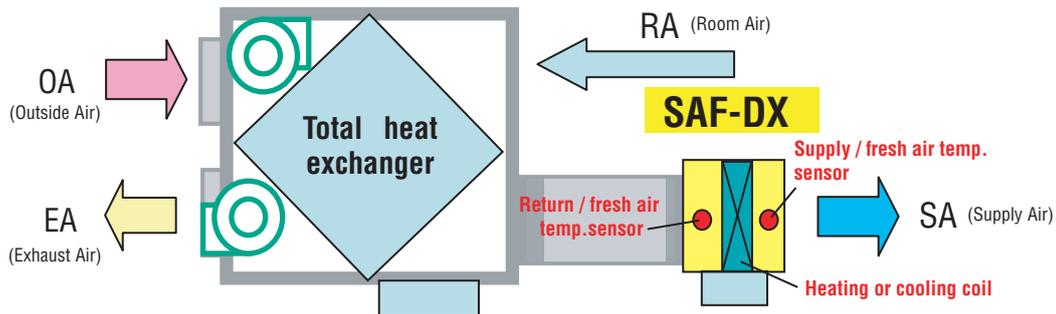
SAF-DX can provide heating or cooling to the fresh air supplied through a 3rd party air handling unit or total heat exchanger such as our SAF series.
