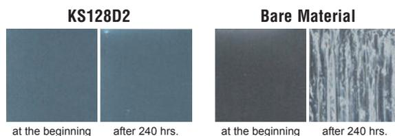
For outside sheet metals, Cation electrodeposition coating is used for undercoat plus polyester powder coating or acrylic baked coating for top coat and corrosion protection is applied for heat exchanger, welded parts, fan guard, fin guard and other major parts.
