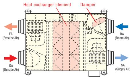
Principle of operation (simple ventilation)
