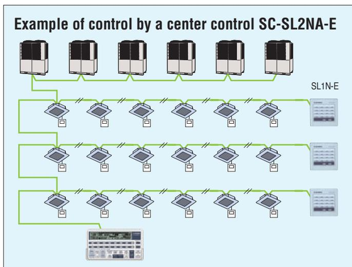
An SC-SL2NA-E performs the start/stop control, monitoring and mode setting of up to 64 units. It is a high quality air conditioner control system that allows up to 64 indoor units to be freely grouped into 1 to 16 groups.
