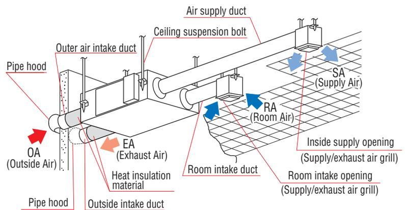
Note: An inspection port is needed for cleaning the heat exchanger and filter 1 or 2 times a year.
