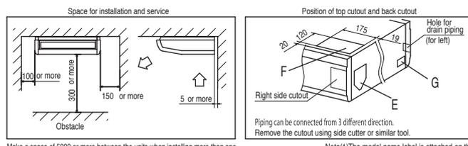
Make a space of 5000 or more between the units when installing more than one.
