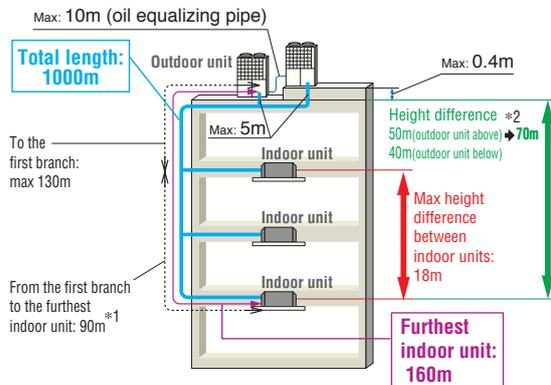
\*1 The difference between the longest and the shortest indoor unit piping from the first branch must be within 40m. (MAX85m)
