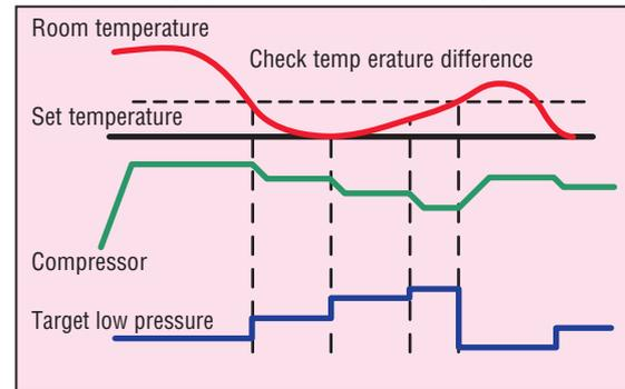
For example, in partial load conditions where you have low cooling and heating requirements, VTCC reduces the compressor frequency and controls the actuators in the outdoor unit. Overall with the VTCC functionality you will always have an additional energy saving of up to 34% (depending on configuration and usage of system) in low cooling and heating load requirements.
