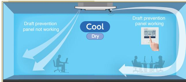
User can position Draft Prevention Panel panels by using the remote controller only (RC-EX3, RCN-T-5AW-E2).
