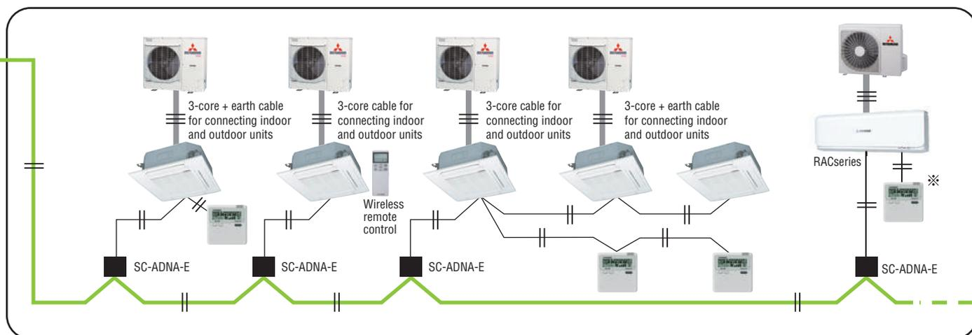
※ SC-BIKN is necessary to connect to wired remote controller.
