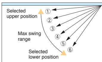
※The wireless remote control is not applicable to the Individual flap control system.
