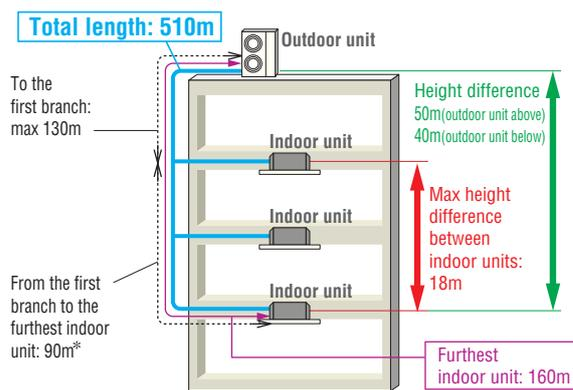
\* The difference between the longest and the shortest indoor unit piping from the first branch must be within 40m.
