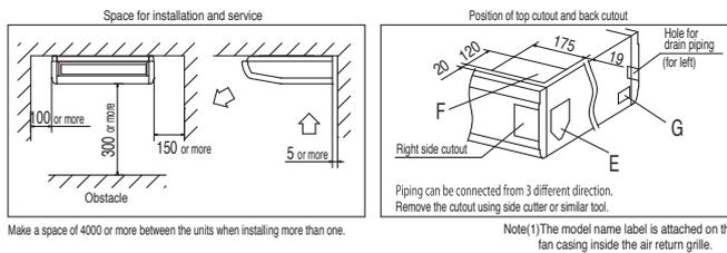
Make a space of 4000 or more between the units when installing more than one.
